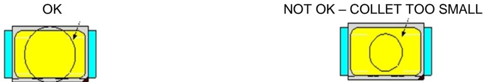
Setting the height of the collet is crucial in order to avoid damage to the top view SMD. If the collet setting is set to too low of an altitude, the collet will press down on the SMD, causing damage or breakage to the encapsulant and cause distortion or breakage of the gold wire.
